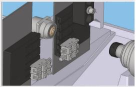
The virtual programming station is more than CAM system. It includes the 3D virtual machine for the configuration of tools and tool holders, a perfect first step program to prepare your complex jobs and all possible cycles and synchronizations for programming complex parts. ESPRIT CAM technology creates optimized toolpaths and safe links. In combination with certificated postprocessors your job is running on the machine as soon as possible.
